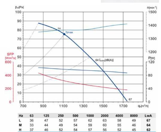
Test standard: ISO 5801 Fan tested without guard and with bellmouth entry
